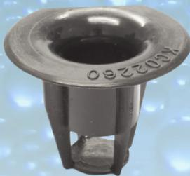
EVX nozzles are gravity fed nozzles used in EVAPCO AQXS and AQXD crossflow cooling towers, the EVX nozzle is manufactured from durable PVC. The EXV design utilizes holes drilled in the hotwater basin where the nozzles are then press fit into position, this design ensures nozzles do not work loose under the force of water entering the hot water basins of larger crossflow cooling tower designs.
